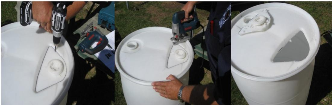
3. Drill a hole (with a 1 3/4" hole saw or 1 3/4" paddle bit) at the top of the barrel for an overflow and one at the bottom of the barrel for the spigot. If barrel will not be elevated locate hole for spigot high enough to attach hose without crimping.
